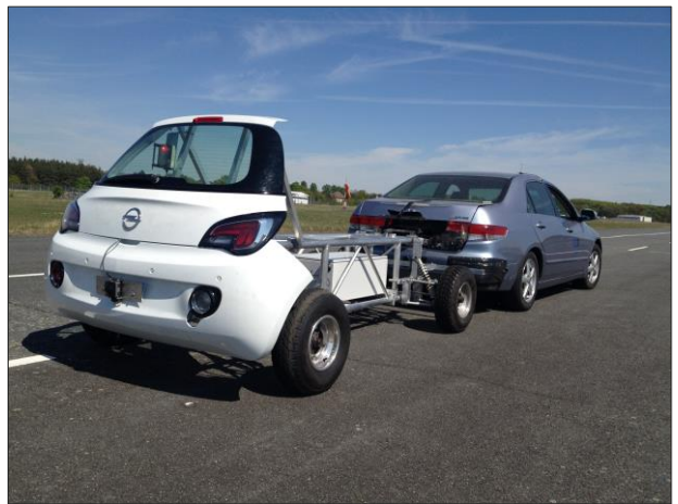
Experimental vehicle for unexpected target approach (EVITA 2.0) of the TU Darmstadt
