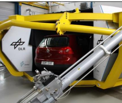
Figure 2. Driving simulator used in the two studies. © DLR
