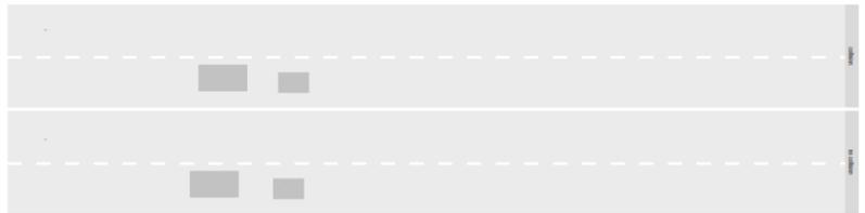
Figure 3. Cut-in scenario: ego speed = 130 km/h; relative speed = 50 km/h. One case with a collision (top) and one case without collision (bottom).
