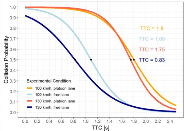
Figure 9. Relationship between collision probability and TTC in form of a logistic regression. The threshold of human performance in each scenario is defined as the inflection point (collision probability = 50%) of the curve.
