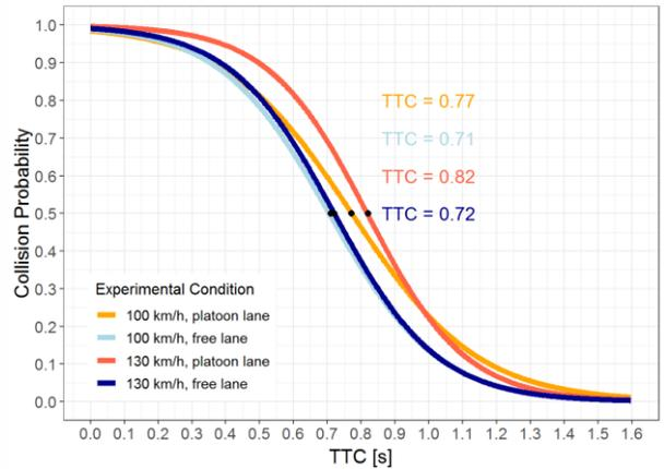
Figure 7. Relationship between collision probability and TTC in form of a logistic regression. The threshold of human performance in each scenario is defined as the inflection point (collision probability = 50%) of the curve.
