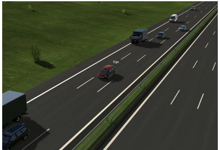
In this scenario the lane markings are missing (e.g. due to a cleared construction side). While human drivers are able to cope relatively easy with this situation, a HAD-F may not.
