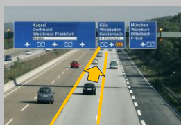
Correct distance to ahead driving traffic Not leaving Ego lane (except for a lane change)
