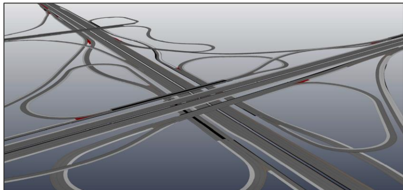
Exemplary visualization of a highway intersection after the surveying and data processing into the output format OpenDRIVE.
