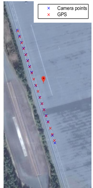
Satellite image of proving ground in Ehra. Plotted is the estimated position of one vehicle according to cameras and dGPS data.
